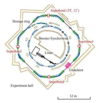
Figure 3: A 1.2GeV low energy compact light source CJSRF [12] is completed in Nagoya.
