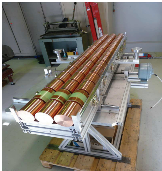
Figure 1: Target with 3 assemblies, each with 15 copper cylinders. The aluminium enclosure and caps are not shown.
