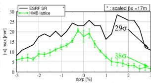
Figure 2: Dynamic aperture of the new lattice compared to the present one.
