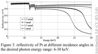
Figure 3: reflectivity of Pt at different incidence angles in the desired photon energy range: 6-30 keV.
