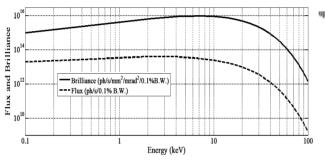
Figure 1: Photon flux and brilliance of ILSF BM source versus energy at I=400 mA and horizontal divergence of 1.5 mrad.
