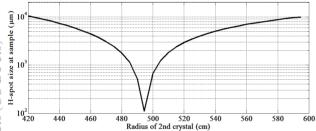
Figure 5: Variation of horizontal (H) spot size at sample position versus 2nd crystal radius.
