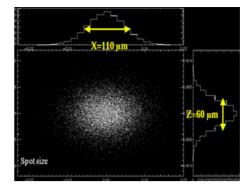
Figure 6: Distribution of photons at sample position (8 keV). The FWHM of the spot size is indicated in the figure.
