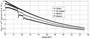
Figure 7: Photon flux after Be window, M1 and M2 mirrors in 6-25 energy range.
