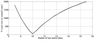
Figure 4: Variation of vertical (V) spot size at sample position versus last mirror radius.
