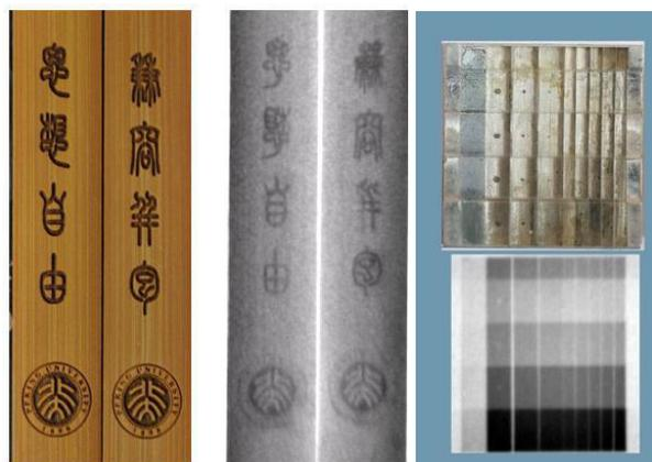
Figure 6: Examples of neutron radiography.
