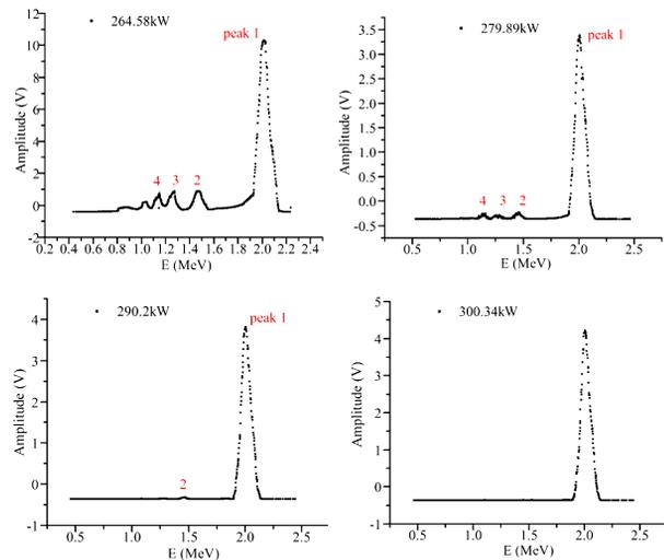
Figure 5: Output deuteron energy spectrum at different RF power.
