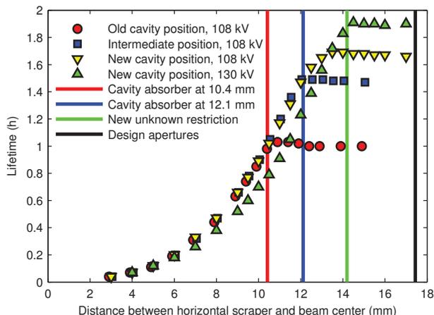
Figure 4: Horizontal scraper measurements for the old, intermediate and new cavity position. The error of the measured lifetime is estimated to be smaller than  $\pm 0.3\%$ . The uncertainty in the location of the beam center is estimated to be  $\pm 0.2$  mm.
