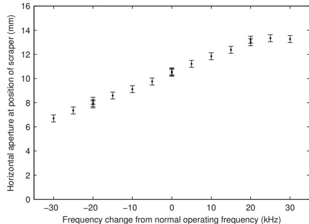
Figure 1: Distance between the beam center and the horizontal scraper position where an effect on the lifetime starts to appear as a function of RF frequency change.
