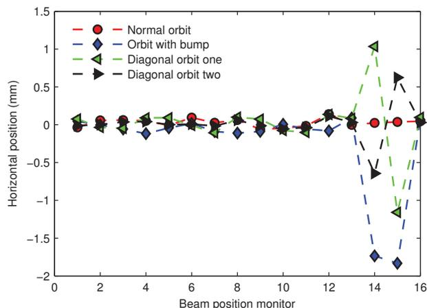
Figure 2: Horizontal beam position at the 16 beam position monitors in MAX III for four different orbits. The error of the measured beam position is estimated to be  $\pm 0.05$  mm.
