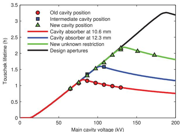
Figure 5: Measurements of the Touschek lifetime as a function of the main cavity voltage for the old, intermediate and new cavity position. The error of the measured Touschek lifetime is estimated to be  $\pm 1\%$  or smaller.
