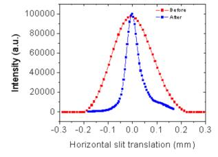
Figure 7: Comparison of the horizontal beam profile before and after the upgrade measured at one user beamline showing the factor of three improvement in brightness (vertical scale is renormalized).
