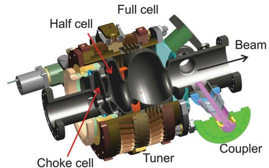
Figure 1: Drawing of the SRF photo-injector cavity with the cavity, beam tube, choke cell and cathode insert in silver grey. Also shown are ancillary components such as the helium vessel, blade tuner, stiffening ring and CW-modified TTF-III coupler.
