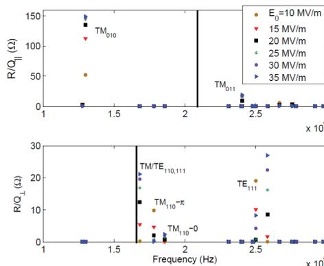
Figure 7: Longitudinal and transverse  $R/Q$  for different peak on axis fields  $E_0$  obtained by integrating the Lorentz forces in steps with respect to  $t = z/(\beta(t)c)$ . The black lines denote the  $TE_{11}$  and  $TM_{01}$  cutoffs of the beam tube.
