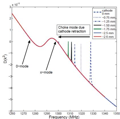
Figure 6:  $D(k^2)$  function of Superfish showing the  $TM_{010}$  monopole passband and the resonance of the choke structure, which varies with the cathode position. At -2.6 mm position the  $\pi$ -mode and choke mode overlap.
