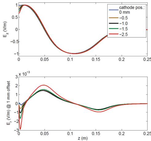
Figure 3: Longitudinal electric field component at  $r=0$  and radial electric field at  $r=1\text{mm}$  versus  $z$  for different cathode positions.
