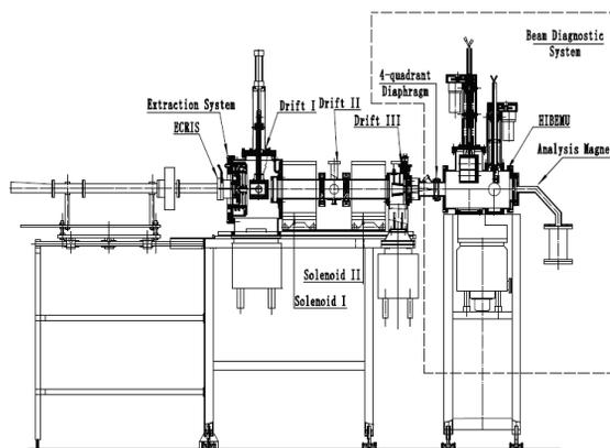
Figure 2: Injector with beam diagnostic system.
