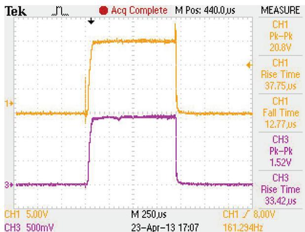
Figure 6: ACCT(CH1) and Slit Cup(CH3) signals.
