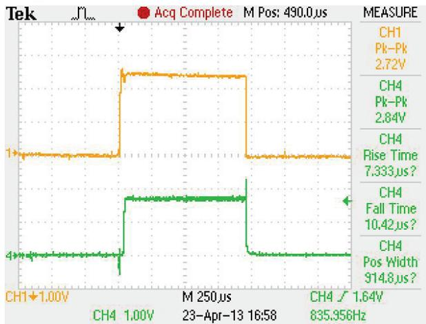
Figure 5: Microwave(CH1) and FC(CH4) signals.
