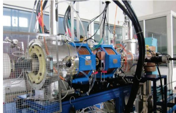
Figure 3: Injector with beam diagnostic system.
