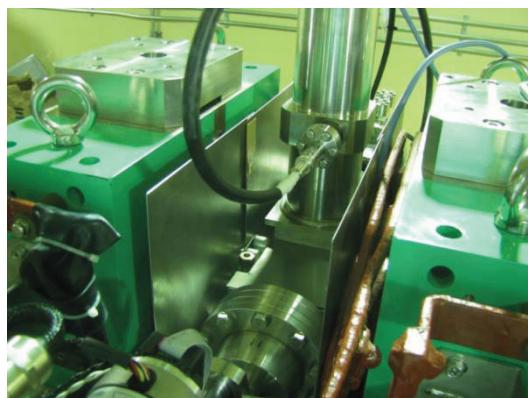
Figure 4: View of magnetic shield installed between the body and coil and on the body surface.
