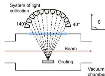
Figure 1: Smith Purcell radiation first generation monitor scheme.
