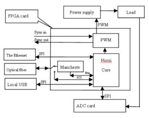
Figure 1: Block diagram.
