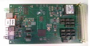
Figure 2: FPGA card.
