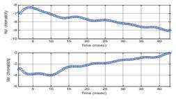
Figure 9: Measured uncompensated chromaticity.
