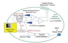
Figure 5: Functional block diagram of the new tune monitor for TLS booster.
