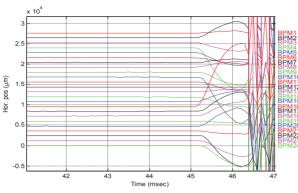
Figure 2: Horizontal beam position variation during beam extraction bumper magnets triggered.
