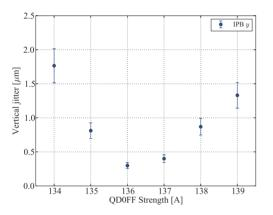
Figure 7: IP waist position scan, around IPB, using QD0FF current.
