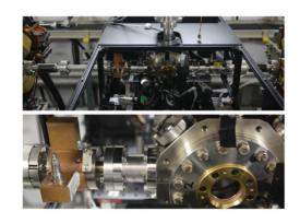
Figure 4: Top : Photo of MFB2FF region, showing the laserwire system from the surrounding quadrupoles (QM14FF and QM13FF). Bottom : Zoom of the laserwire interaction chamber and down-stream BPM, MFB2FF.
