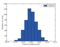
Figure 5: MFB2FF vertical position residual histogram for 500 ATF2 machine pulses.
