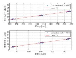
Figure 8: Vertical position correlation between MFB2FF and IPA (top) and IPB (bottom).
