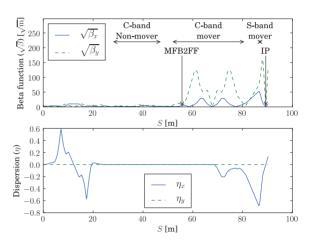
Figure 1: ATF2 beta ( $\beta$ ) and dispersion ( $\eta$ ) as function of distance along the beam line *s* from the first extraction kicker, calculated using MAD version 8 [1].
