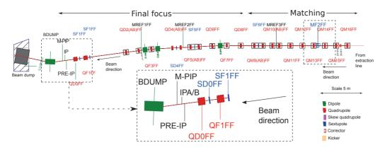
Figure 3: Layout of the ATF2 from the  $\beta$  matching section onwards to the IP and dump. The IP region is zoomed [5].
