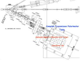
Figure 1: The PEPPo line arrangement terminated by the Compton transmission polarimeter.
