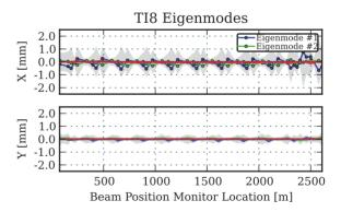
Figure 5: The plot shows the observed (grey) and calculated trajectory variations in TI 8 after the technical stop.
