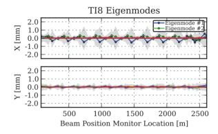
Figure 4: Trajectory variations for TI 8 before the technical stop are shown. In the horizontal plane there are large variations coming from two independent sources.
