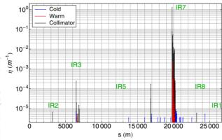
Figure 2: Loss map from SixTrack simulation at 2 TeV.
