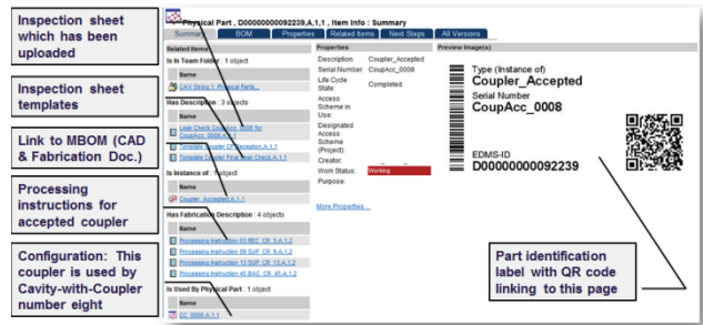
Figure 4: Example physical part record of a coupler during assembly to an accelerator module.
