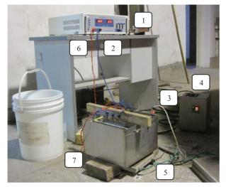
Figure 5: Photo of the improved electropolishing device
