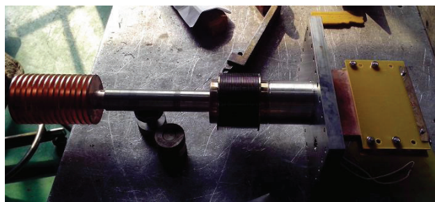
Figure 4: Brazing structure of scraper assemble.
