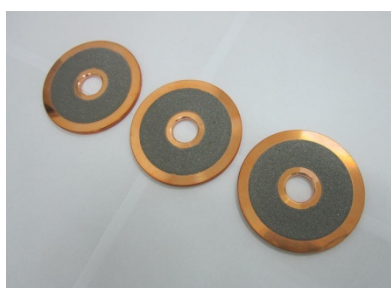
Figure 2: Disks coated with Kanthal.
