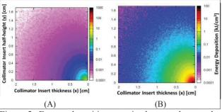
Figure 2: Energy deposition cuts in the x-y plane at the location of  $T_{max}$  in z. (A) 1 nominal bunch of lead ions  $(7\times10^7 \text{ ions, } 2759 \text{ GeV/n})$  with  $T_{max}$  occurring at z = 6.5 cm. (B) 1 nominal bunch of protons  $(1.15\times10^{11} \text{ p})$  at 7TeV with  $T_{max}$  occurring at z = 7 cm.
