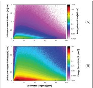
Figure 3: Energy deposition cuts in the x-z plane at collimator insert half-height (plane of symmetry). (A) 1 nominal bunch of lead ions  $(7 \times 10^7 \text{ ions}, 2759 \text{ GeV/n})$ . (B) 1 nominal bunch of protons  $(1.15 \times 10^{11} \text{ p})$  at 7TeV.
