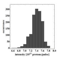
Figure 4: Beam position and pulse intensity stability during a 48 hour run (1500 extractions) for the HRMT01 experiment. The beam position has a  $\sigma$  of 0.3(0.1) mm in the horizontal(vertical) plane, and the beam intensity is stable to 1% level.
