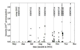
Figure 1: 2012 time-line of the HiRadMat experiments. The labels indicate the nine experiments of the year following the initial setup period. The maximum pulse intensity of  $3.3 \, 10^{13}$  protons was achieved.
