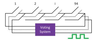
Figure 4: Beam Permit Loop.
