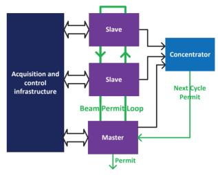
Figure 6: Interlock System prototype synopti.c
