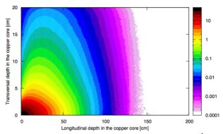
Figure 2: Energy deposition inside dump (GeV/cm<sup>3</sup>)
