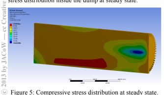
Additionally, peaks of 60 MPa are produced by the dynamic effect of each pulse hitting the dump, resulting in a total stress of 100 MPa. It should be noted that the dynamic loading plays an important role as the pulse period could be as high as 2.4s over several days (especially during commissioning). In other words, the loading could reach a 1E6 cycles over one month only.
