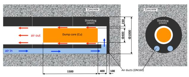
Figure 3: Proposed design for new dump-shielding assembly
