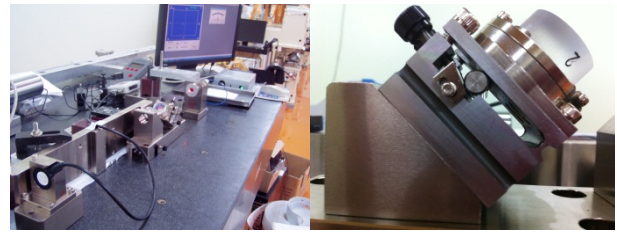
Figure 3: Illustration of PSD adjusting mechanism.
