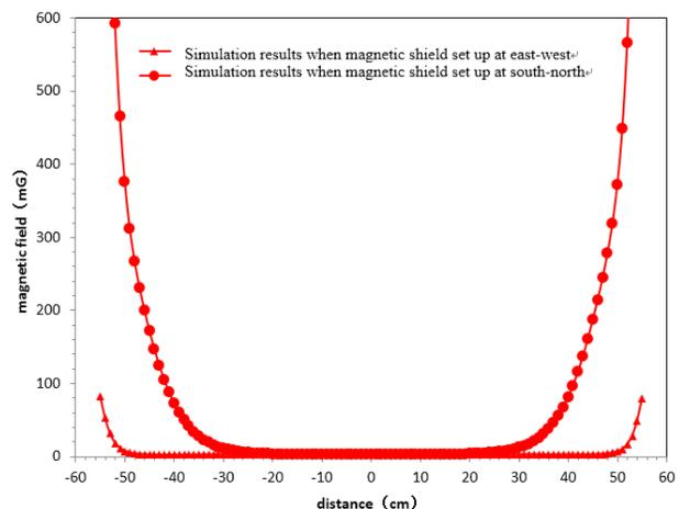
Figure 5: Simulation results when the magnetic shield setup at east-west direction and south-north direction at 4.2K
