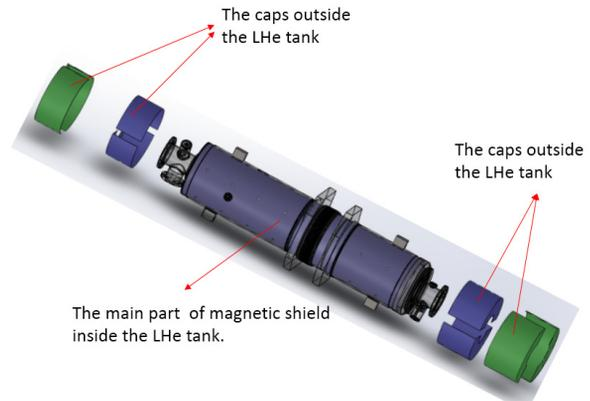
Figure 2: Schematic diagram of the magnetic structure
