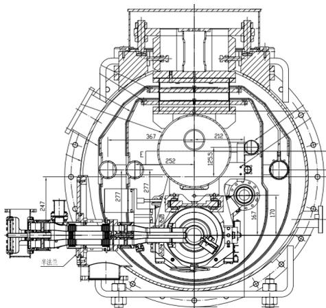
Figure 1: Schematic view of the cryomodule cross-section at IHEP.
