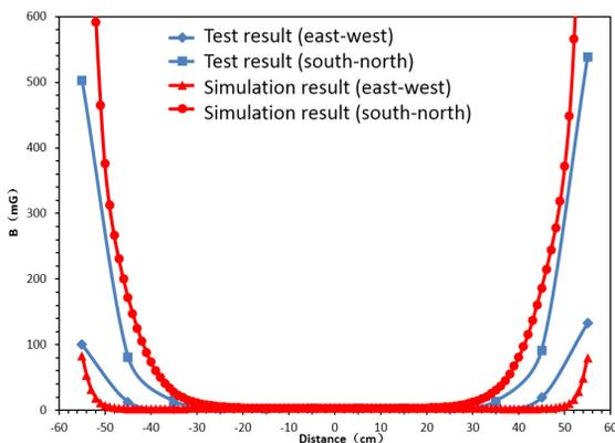
Figure 7: Test results and the simulation results of magnetic shield at room temperature
