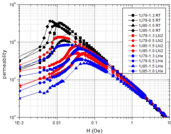
Figure 4: Permeability characteristics of different material at room temperature (RT), liquid nitrogen temperature (LN2), and liquid helium temperature (LHe), respectively.
