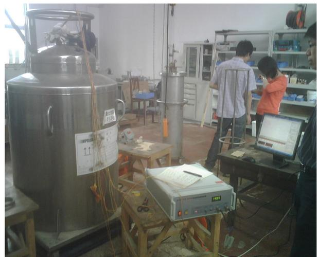
Figure 3: The photo of the permeability measurement experiment at LHe temperature.
