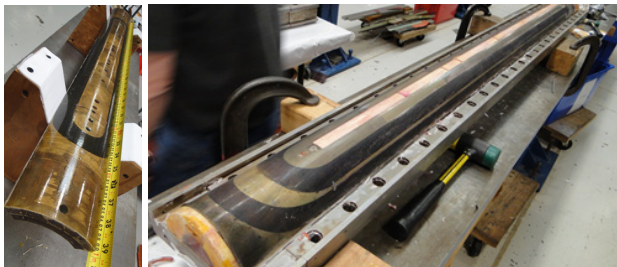
Figure 2: The 1 m long quadrupole coil (left) and the 2 m long dipole coil (right) impregnated with Matrimid.
