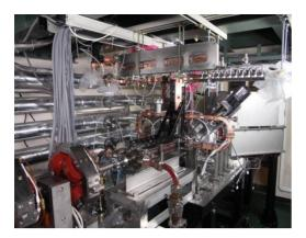
Figure 2: 30 MeV X-band (11.424GHz) Electron Linac.
