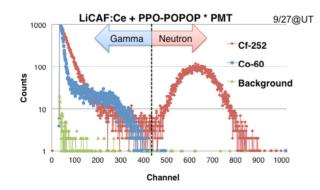
Figure 7: Signals from for Neutrons from Cf-252 and  $\gamma$ -rays from Co-60.
