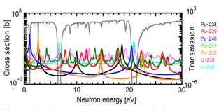
Figure 9: Expected Neutron Transmission Result by Using the Precise Nuclear Data.
