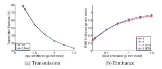
Figure 8: Transmitted current and emittance as a function of input emittance for 60 mA beam using emittance ellipse shown in Fig. 7.
