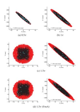
Figure 2: Beam profiles and horizontal emittance distributions for RFQ transmission simulations using the matched Twiss parameters. Captions indicate the normalised *rms* input emittance: see Fig. 1 for particle colouring.
