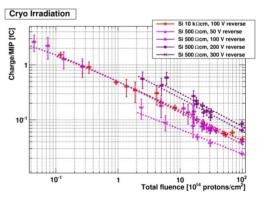
Figure 3: Dependence of the charge collected in Si detectors with a resistivity 500 cm on fluence.
