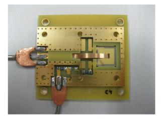
Figure 2: Holder for direct current readout from Cividec.
