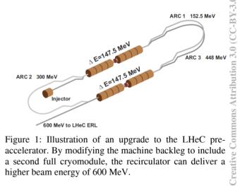
Figure 1: Illustration of an upgrade to the LHeC preaccelerator. By modifying the machine backleg to include a second full cryomodule, the recirculator can deliver a higher beam energy of 600 MeV.
