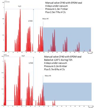
Figure 2: Outgasing of EPDM valves used on the power couplers before and after baking. Blue zone show pollutants above specifications.
