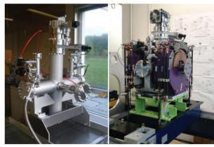
Figure 3: Inter-cryomodules warm sections during clean room assembly (left) and on alignement bench (right).
