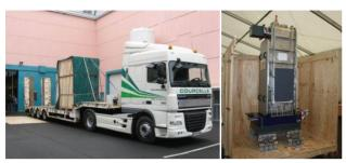
Figure 4: Transportation test of the cryomodule CMA2 from Saclay to GANIL. Right picture shows the cryomodule inside his crate, fixed on its damping support.
