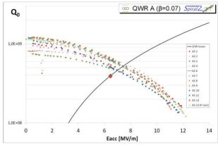
Figure 1:  $Q_0$  vs.  $E_{acc}$  curves of  $\beta$ =0.07 cavities.
