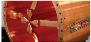
Figure 4 : RFQ end-vane details.
