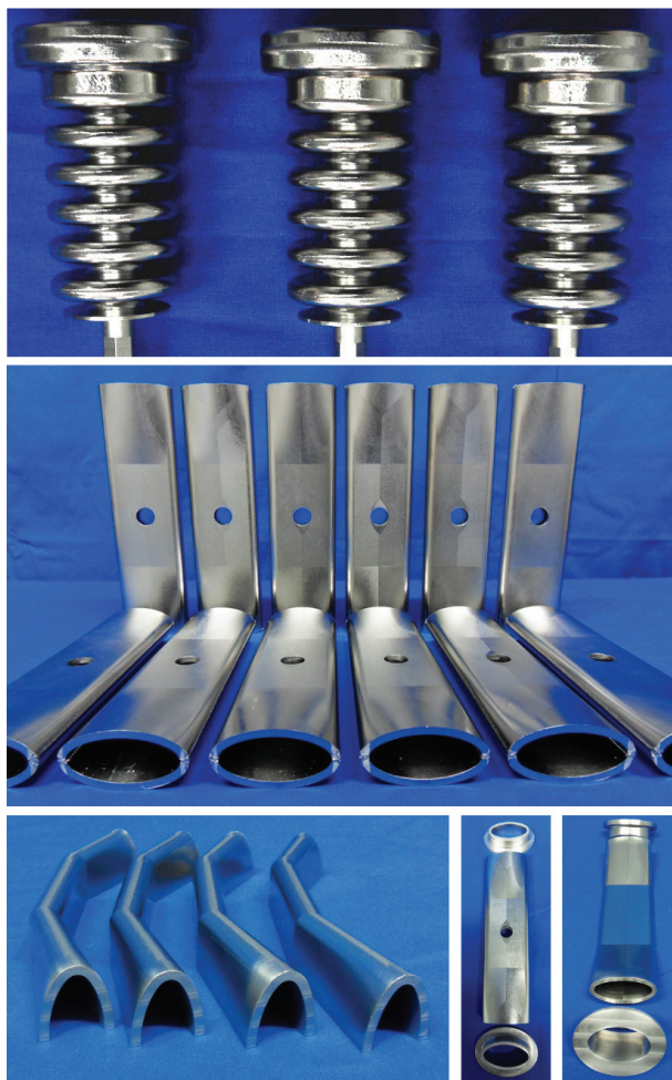
Figure 3: Production status of the dynamic bellow tuners (top), the straight stems (middle), and the inclined end stems (bottom).
