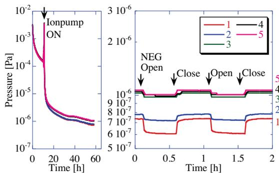
Figure 3: Evacuation curve and change of vacuum pressures caused by the NEG pumps (configuration #2).
