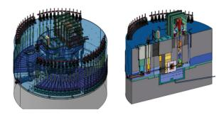
Figure 3: Monolith layout. Left: Perspective view. Right: Side view along the vertical plane of the proton beam.
