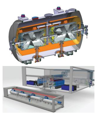
Figure 6: Top: A cryomodule with 2 double spoke cavities. Bottom: Medium- $\beta$  cryomodules with 4 elliptical cavities connect through a waveguide stub to the RF gallery.
