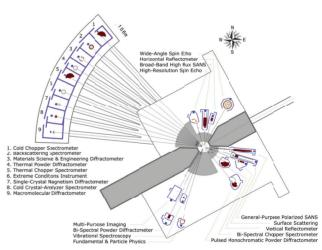
Figure 2: Neutron beamlines and instruments in the reference instrument suite that is used for illustrative purposes.
