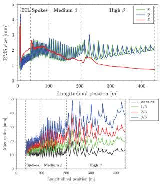
Figure 8: Top: RMS beam sizes from the MEBT to the end of the high- $\beta$  section. Bottom: Maximum beam radius versus distance with increasing errors. Black, green, red and blue curves, respectively, represent error amplitudes at 0/3, 1/3, 2/3 and 3/3 of full strength.
