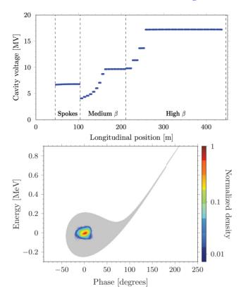
Figure 7: Top: Cavity voltage versus distance along the linac. Bottom: Longitudinal acceptance, referred to the entrance of the DTL. The actual beam out of the MEBT is represented by the coloured distribution at the centre.
