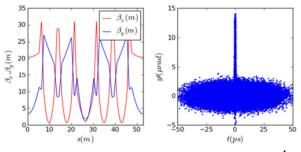
Figure 3: Left: NSLSII lattice. Right: phase space y', y
