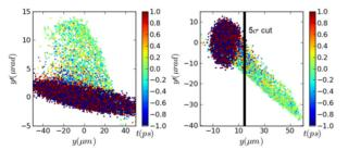
Figure 4: Phase space of y', y at crossing point and radiator respectively.
