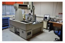
Figure 2: Picture of Mitutoyo 3D machine (precision and resolution of  $5/1\,\mu$ m) used for dimensional testing, with the chamber body and special BPM positioning tool at the edge.
