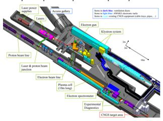
Figure 3: Integration of the AWAKE experimental components in the experimental area.
