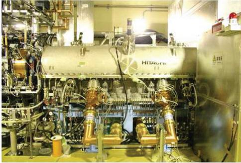
Figure 4: A radio-frequency quadrupole.
