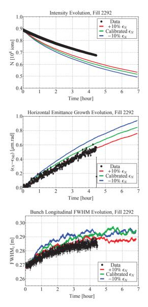
Figure 4: Evolution of a singe bunch compared to simulation. Top: intensity, middle: emittance, bottom: longitudinal FWHM.
