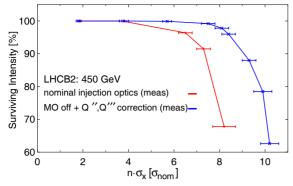
Figure 3: Surviving beam intensity 30 seconds after a transverse kick versus the kick amplitude before (red) and after correction (blue).
