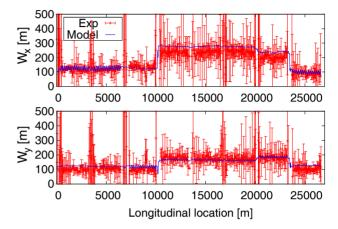
Figure 5: Chromatic  $\beta$ -beating (Montague function) for the nominal LHC optics at  $\beta^*=0.4$  m compared to the model prediction (blue line).
