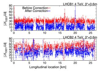
Figure 6: First chromatic coupling correction in the LHC for Beam 1 (top) and Beam 2 (bottom).
