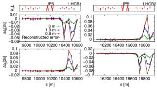
Figure 1: Illustration of the segment-by-segment technique applied to IR5 simultaneously to the two beams and three different  $\beta^*$ . The black lines show the reconstructed error model.
