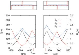
Figure 1: First arc cell on either side of IP1 in the present LHC for Beam 1. Dipoles are shown in blue and quadrupoles in red.
