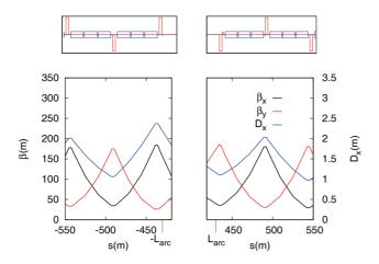
Figure 2: First arc cell on either side of IP1 in the present LHC for Beam 2.
