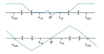
Figure 4: Sketch for the conditions over dispersion matching: (11) [top] and (12) [bottom].
