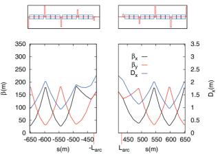
Figure 5: Modified optics of the two first arc cells on each side of the IP (Beam 1), for matching to a symmetric IR optics.
