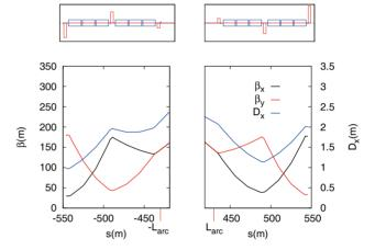
Figure 3: Modified optics of the first arc cell on each side of the IP (Beam 1), for matching to a symmetric optics.
