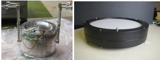
Figure 8: LH 2 absorber (left) and LiH disk (right).
