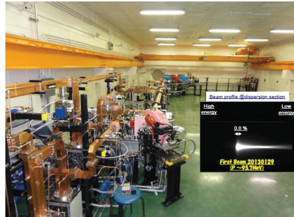
Figure 2: Photograph of new injector linac and the beam profile of first accelerated beam at dispersion section.
