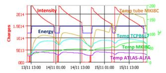
Figure 1: Measured LHC beam intensity (red) and energy (dark blue), along with the measured temperatures of the ceramic tube of the injection kicker MKI-8C (orange), of the skew primary collimator TCP.B6L7.B1 (light blue), of the magnet ferrite of the injection kicker MKI-8C (green) and of the ATLAS-ALFA detector (purple).
