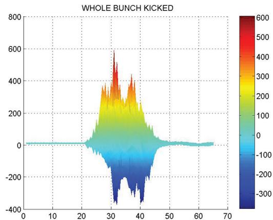
Figure 5: Projection of the bunch oscillations over time to the longitudinal bunch coordinate for the whole-bunch-kicked case.
