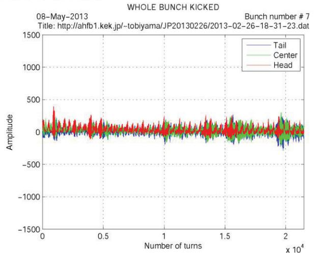
Figure 4: Time evolutions of the oscillations of the head, the center and the tail of the bunch over 22,000 turns, when the whole bunch is kicked by the iGp12 module.
