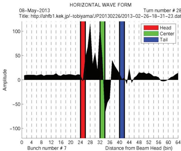
Figure 2: Snapshot of typical intra-bunch oscillation sampled at the rate of RF frequency times 64.
