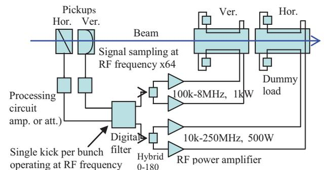
Figure 1: Schematic view of the present transverse bunch-by-bunch feedback system in a narrowband mode.
