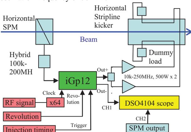
Figure 3: Measurement setup of the intra-bunch feedback system with the iGp12 module.
