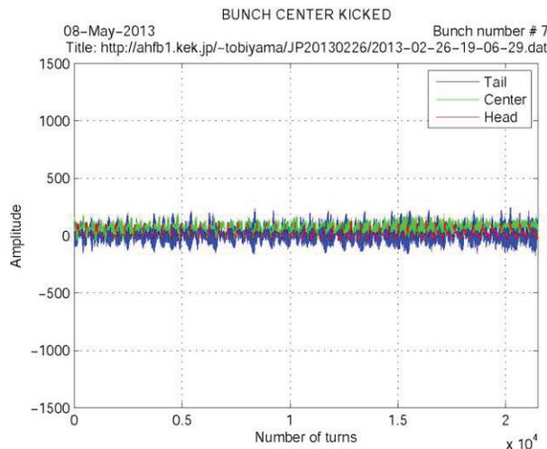
Figure 7: Time evolutions of the oscillations of the head, the center and the tail of the bunch over 22,000 turns, when only the center of the bunch is kicked.
