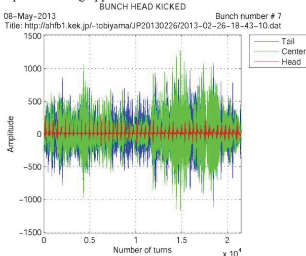
Figure 6: Time evolutions of the oscillations of the head, the center and the tail of the bunch over 22,000 turns, when only the head part of the bunch is kicked.
