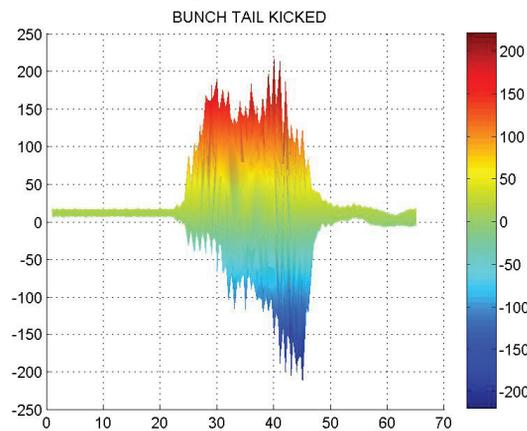
Figure 8: Projection of the bunch oscillations over time to the longitudinal bunch coordinate when only the tail of the bunch is kicked.
