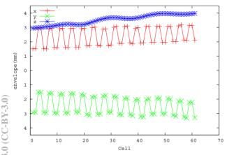
Figure 5: The beam envelope after the equipartitioning optimization with the new method.
