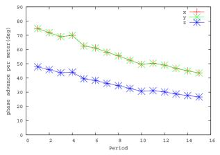
Figure 4: The phase advance after the new "equipartition" optimization.
