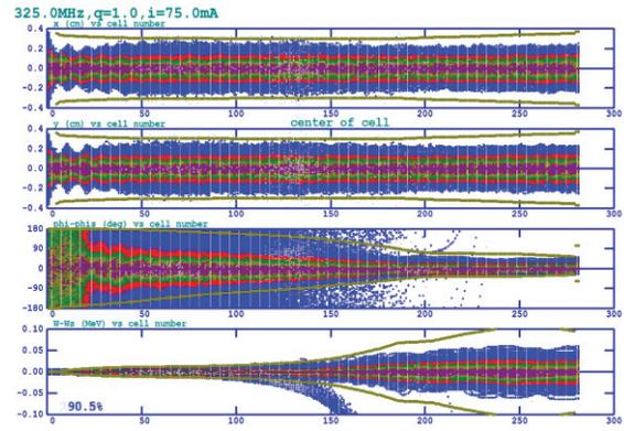
Figure 5: Beam dynamics in the RFQ for the input current of 75 mA, 5000 particles. From top to bottom are: x, y, phi, and energy coordinates versus cell number. The percentage transmission is 90.5%.
