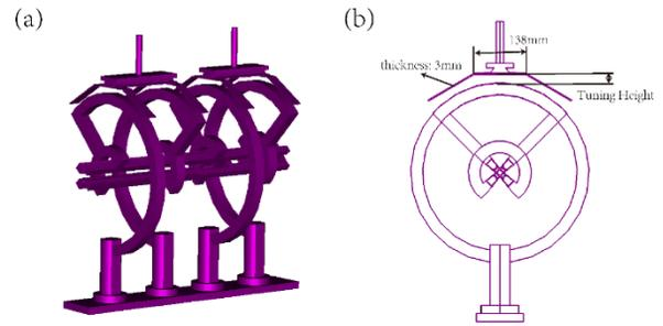
Figure 3: The tuning system in the CRS cavity.
