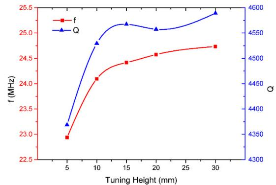
Figure 4: Frequency and Q as a function of tuning height.
