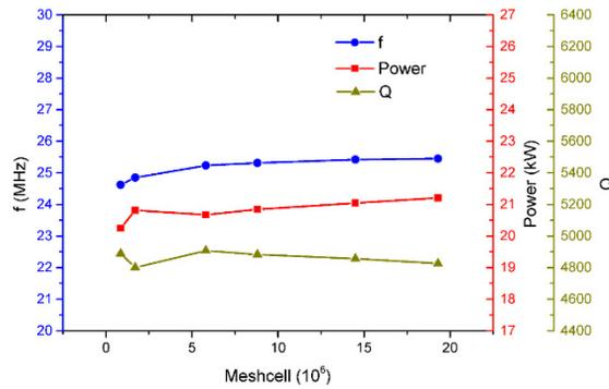
Figure 2: Simulated cavity rf properties via mesh.
