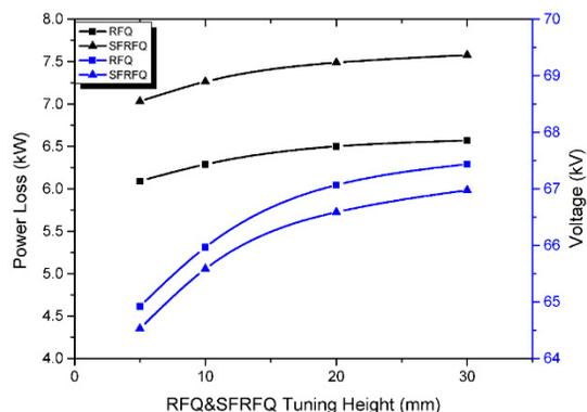
Figure 5: Power loss and inter-vane voltage as a function of RFQ&SFRFQ tuning height.
