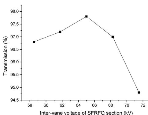
Figure 7: Transmission as a function of SFRFQ inter-vane voltage.
