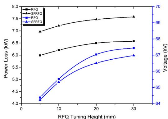
Figure 6: Power loss and inter-vane voltage as a function of RFQ tuning height.
