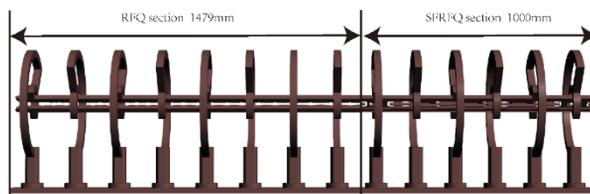
Figure 1: Inter structures of CRS cavity.
